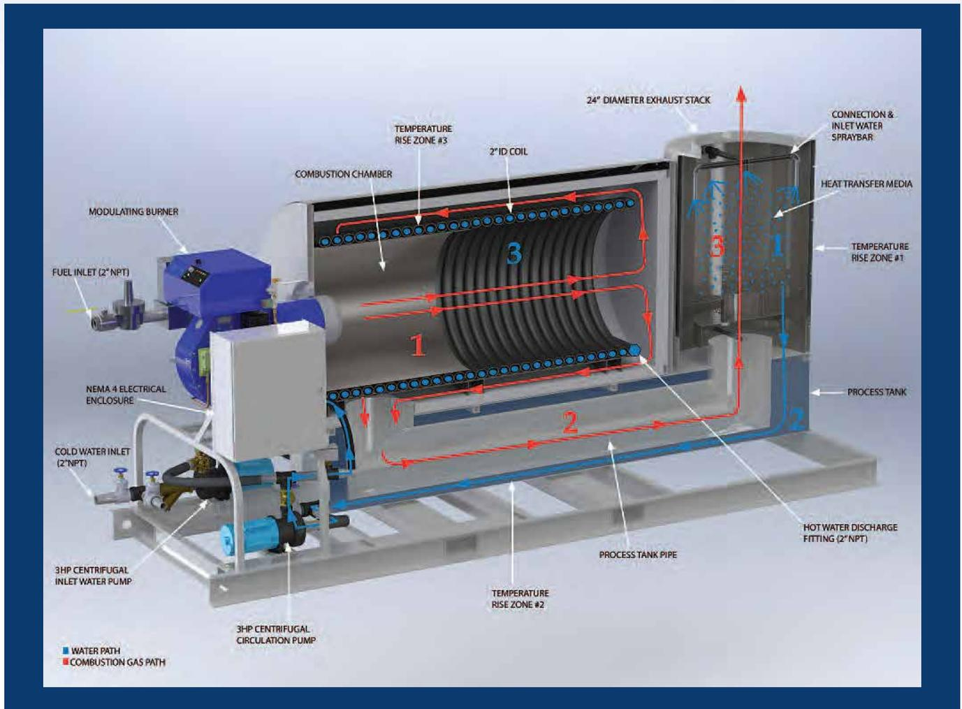
Operation of the Hybrid Heater is fairly simple: Please see the illustration above, and consider the flow of **combustion gas** (in red), and then the flow of **water** (in blue).
