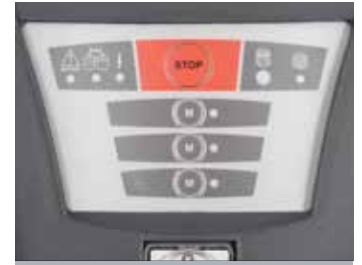
Membrane switch keypad with LED indicators
