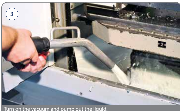
Turn on the vacuum and pump out the liquid.
