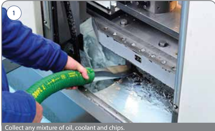
Collect any mixture of oil, coolant and chips.
