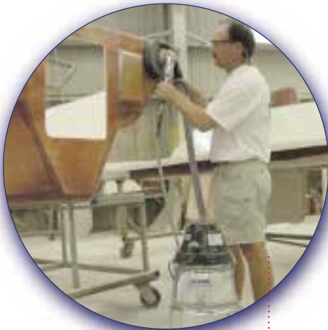
The 811 attached to a grinder for immediate removal of dust.
