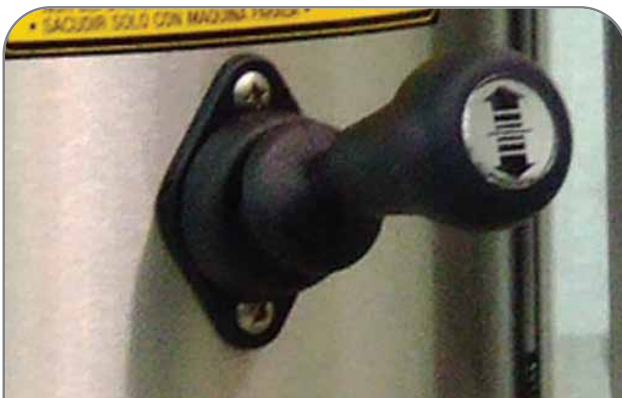
External filter shaker on A15 EXP for dry material collection
