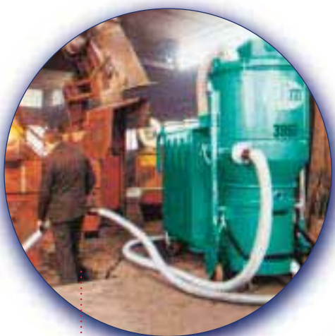
Recovery of sand and gravel in a foundry.
