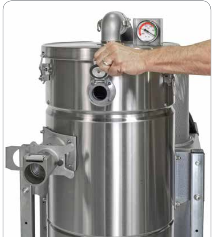
Step 2: Open flap to allow outside air to pass through filter.
