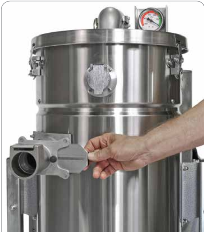
Step 1: Close slide valve on inlet to build vacuum pressure.
