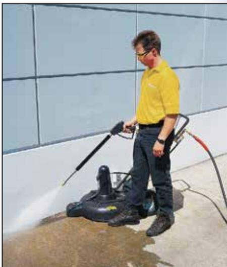
A holster-mounted trigger gun and insulated wand make for convenient spot cleaning of hard-to-reach places.
